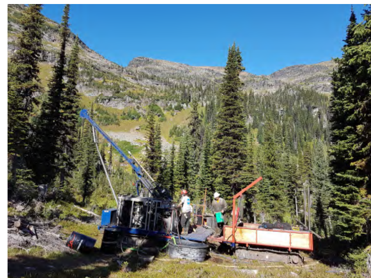
Tracked drill minimizes surface disturbance and tree-cutting
